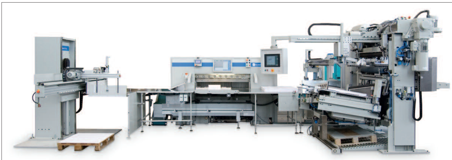
The Baumann-Wohlenberg No 3 cutting system consists of a fully automatic Baumann BASA 3 jogging system with integrated pile logistics, a Baumann BFS-V gripper transport system, a Wohlenberg 132 high speed cutter and a Baumann BA 3 unloader.
