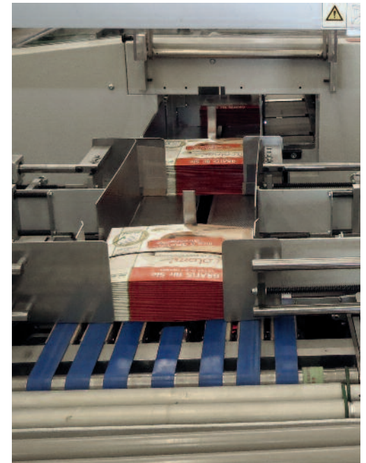
The Cara has a maximum output of one cross-strapped bundle every 1.8 seconds.
