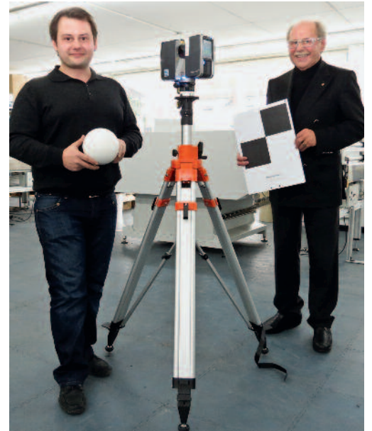
Christian (left) and Peter Hanosek presenting one of their 3D laser scanner from the Faro brand and the “reference points”, which have firmly to be attached overlaying visible to the ceiling of the hall which is to be scanned. The strategic placement of these reference points needs a lot of experience. When scanning a common industrial hall, 10 up to 25 gigabyte of data will be stored on the SD card of the laser scanner.
