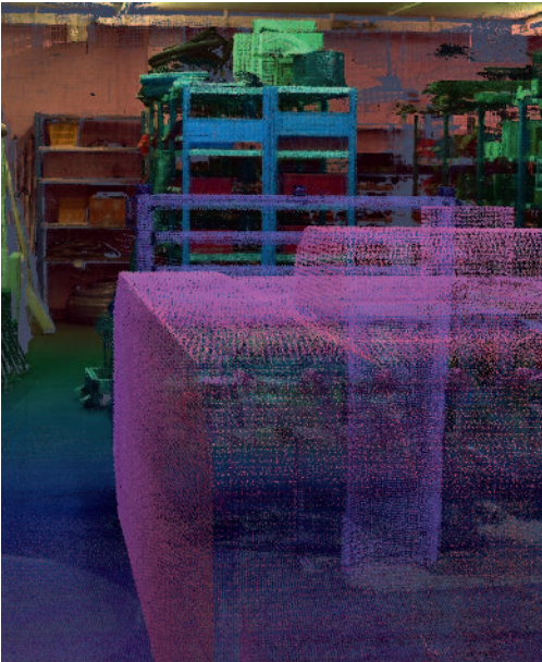
The 3D laser scanner originally generates “black and white point cloud images”. However, these can be augmented with colour information later on due to an implemented camera function.
