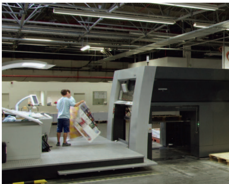
Kodak's thermal CtP systems supply the online printer's large format sheet-fed offset presses with plates.
