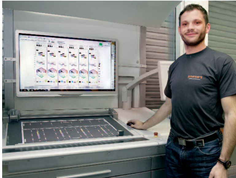
Production Manager Fabio Wellenzohn at the control desk of the press. The measurement and control functions of Ink-Zone Instrument Flight featuring the familiar hexagon chart are visible in the background.
